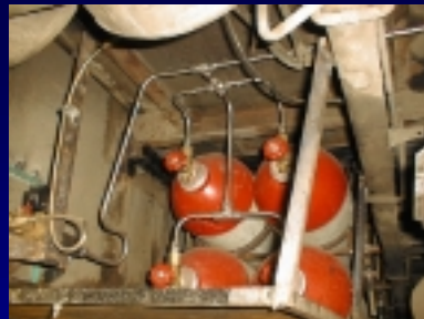
No stress loops / piping too rigid / unsupported piping
