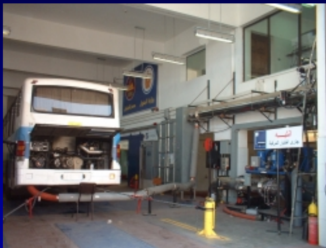
Heavy-Duty Transient Chassis Dynamometer Emission Measurement Facility in Cairo, Egypt
